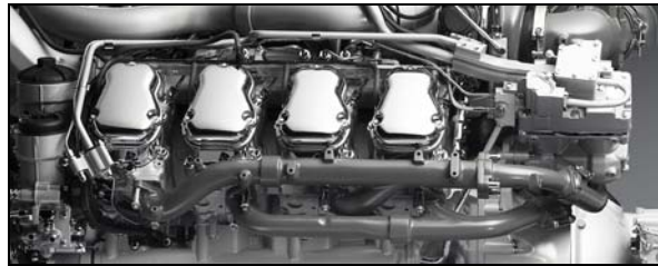
Figure 1 Exhaust collectors of the V8 engine (left bank)
