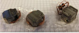
**Figure 6.13.** Attocube ANPx51RES (left and centre) and Attocube ANPz51RES (right) nano-positioners used for scanning and positioning in three dimensions. The small squares on the paper are 5mm, and the positioners have a footprint of 15x18 mm.
