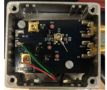
**Figure 4.8.** The error detector (P1). A photo diode (S9055) is soldered directly onto a circuit board (MAX3658A evaluation board). The board is mounted in an aluminium casing and the signal is fed out via SMA-connectors.
