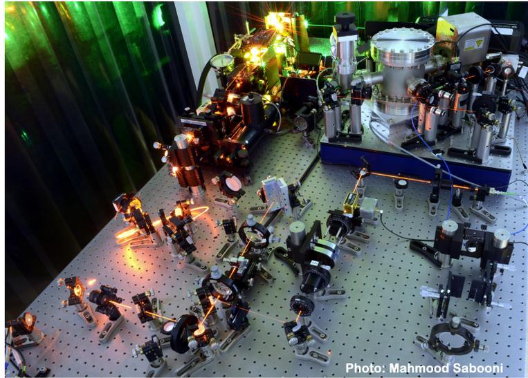
**Figure 4.6.** A picture of the dye laser stabilization set-up. The dye laser is visible in the upper left corner. The vibration isolation platform with the vacuum chamber containing the cavity is standing in the upper right corner.
