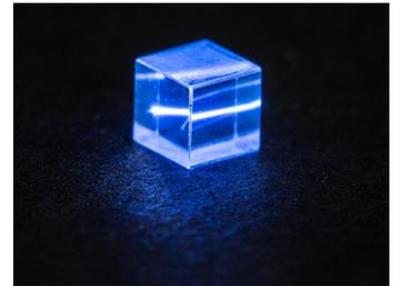
**Figure 7.1.** A 0.088% Ce:Y<sub>2</sub>SiO<sub>5</sub>-crystal fluorescing brightly when excited with a laser beam at 371 nm.
