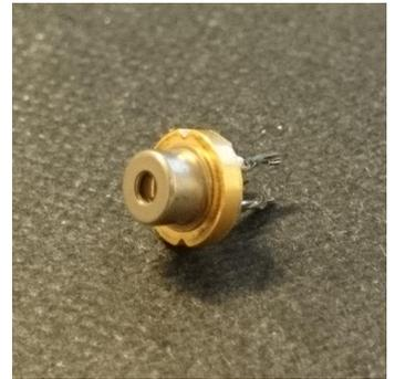
**Figure 5.1.** *The Toptica LD-0375-0020-2 laser diode.*
