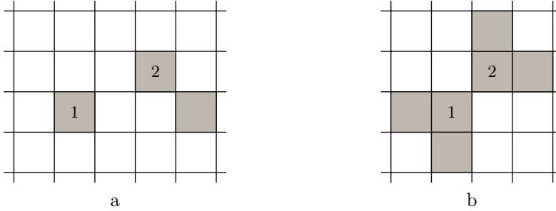
Figure 5: Example of isolated mesh elements (marked “1” and “2” in a) and corner connection (between the non-isolated elements marked “1” and “2” in b) that may appear in a mesh describing a discretized structure. Metallic regions are depicted in gray shading.
