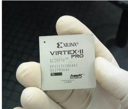
Figure 2.1 An FPGA circuit.
