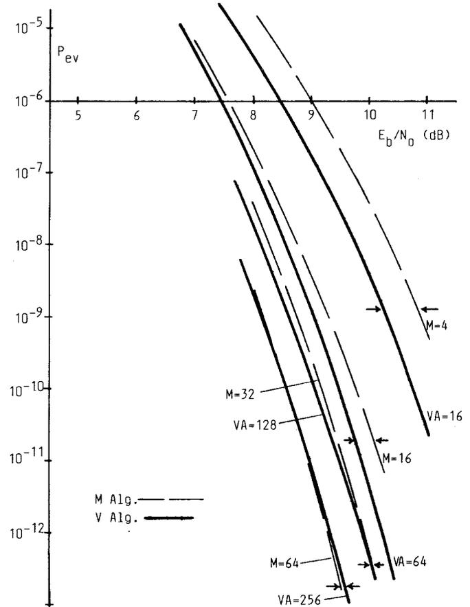
Fig. 8. Counting estimates of the event error probabilities for the  $M$ -algorithm decoding of the ODP feed-forward systematic encoder  $G_{81}$  with  $M = 4, 16, 32$ , and  $64$  and for the four-fold larger Viterbi decoder of sizes  $16, 64, 128$ , and  $256$ . The Viterbi algorithm (VA) encoders are ODP feed-forward nonsystematic with memory  $m = 4, 6, 7$ , and  $8$ . The quarter-size  $M$ -algorithm has lower error probabilities above VA size  $128$ .
