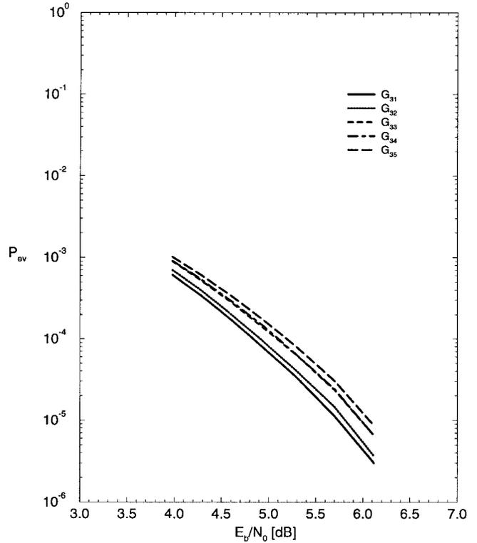
Fig. 3. Simulated event error probabilities observed in tests of a set of systematic encoders, each of whose distance profile  $\mathbf{d}^p$  successively underbounds the others, when decoded with  $M = 32$ . The heavy line is the ODP feed-forward systematic encoder  $G_{31}$  which always performs best.
