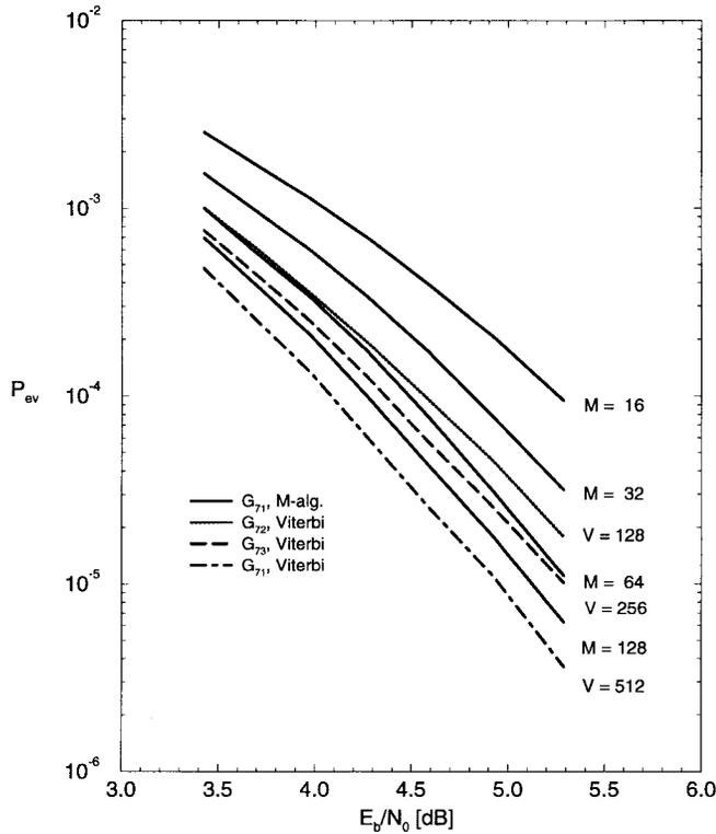
Fig. 7. Observed event error probabilities for a nonsystematic encoder  $G_{71}$  with the  $M$ -algorithm and three different best- $d_{\text{free}}$  nonsystematic encoders  $G_{71}$ ,  $G_{72}$ ,  $G_{73}$  with Viterbi decoders.
