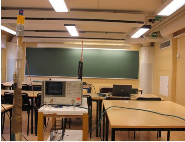
Figure 9.4: Overview of the measured scenario. Tx antenna in front and Rx antenna in the back.
