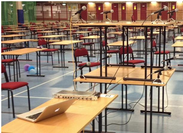
Figure 10.4: Setup for indoor experiment using microphones and distinct manually made sounds.
