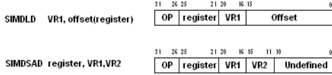
Figure 1. New SIMD instructions are 32-bit and follow the same bit structure as the other processor instructions.
