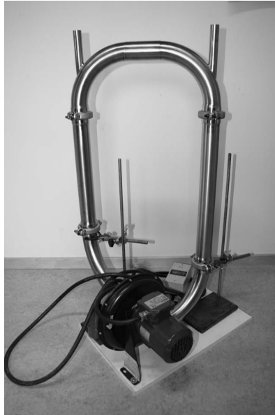
Figure 2.5: The carbon black soot distributor.
