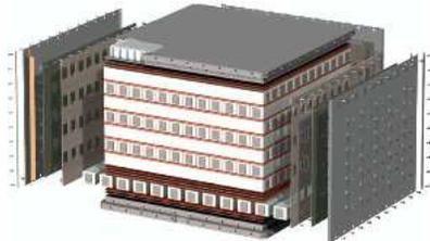
Fig. 1. Each calorimeter tower consists of 8 layers of 12 CsI(Tl) crystals stacked in an  $x$ - $y$  configuration. A calorimeter tower contains 96 crystal logs and measures about  $40 \times 40 \times 20 \text{ cm}^3$ . In total there are 1536 crystals.
