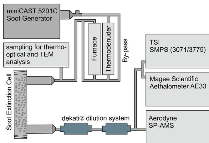
**Fig. 1.** Experimental set-up. The set-up included the soot extinction cell but is not part of the current analysis. Results on optical properties including the soot extinction cell have been published previously [35]. (A colour version of this figure can be viewed online.)
