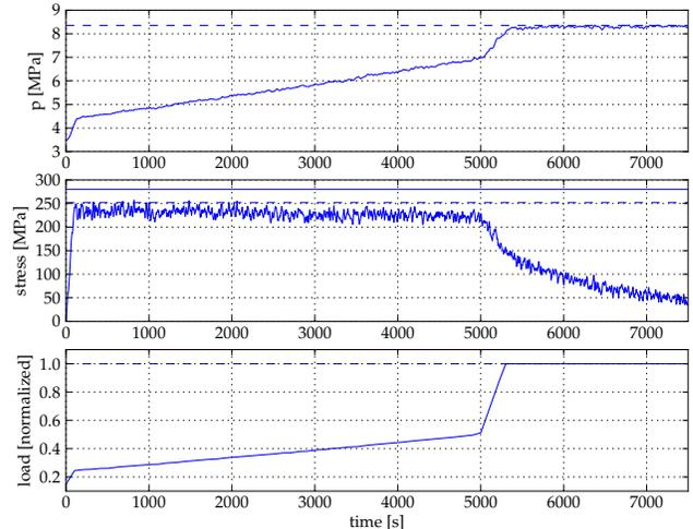
Fig. 2. Closed loop control with NMPC. *Top*: Evaporator pressure  $p$  and reference value  $p_{\text{ref}}$  (dashed). *Middle*: Rotor stress  $\sigma$ , soft constraint (dashed) and hard constraint (solid). *Bottom*: Turbine load  $u$  and upper limit (dashed).
