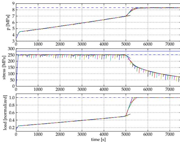
Fig. 3. NMPC iteration results at closed loop control. *Top*: Evaporator pressure  $p$  and reference value  $p_{ref}$  (dashed). *Middle*: Rotor stress  $\sigma$ , soft constraint (dashed) and hard constraint (solid). *Bottom*: Turbine load  $u$  and upper limit (dashed).
