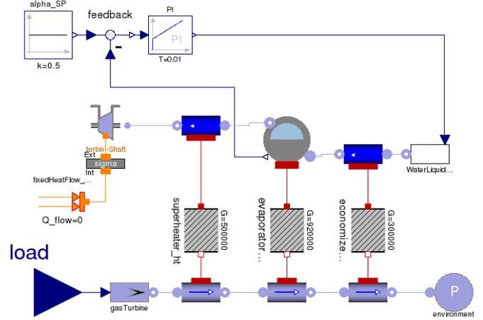
Fig. 1. Object diagram of Modelica plant model.
