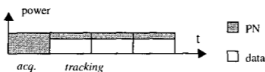
Fig. 2. Structure of the transmitted signal.
