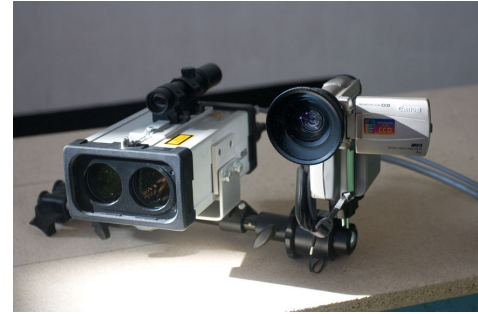
Figure 2: Laser distance meter and video camera for documentation
