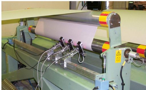
Fig. C9. The crepe-wrinkle detector mounted in a rewinder at a paper mill (left). Typical response due to a large crepe wrinkle (right).
