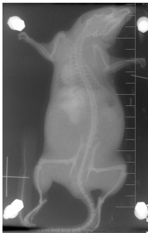
Fig. A10. A one-minute exposure of a sacrificed Wistar-Furth rat. The grey-scale extends from 2 \mu Gy (white) to 13 \mu Gy (black) over 256 levels.
