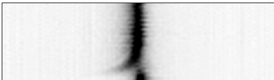
Fig. A17. Laser-induced coherent strain wave propagation into an InSb crystal.
