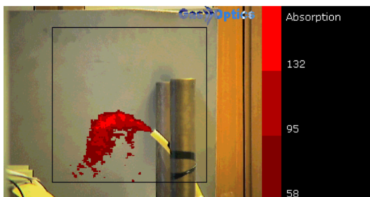
Fig C6. Gas correlation imaging of a sulphur hexafluoride flow.
