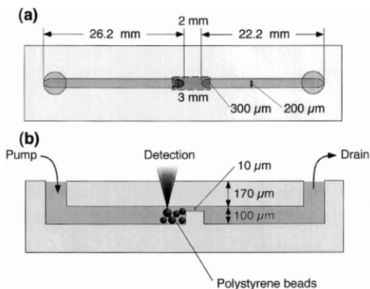
*Figure 12. Quartz glass microchip for polystyrene bead-based immunoassay. The analyte (secretory human immunoglobulin A, s-IgA) was adsorbed on the beads followed by recognition with gold-labelled antibodies monitored by thermal lens microscopy (TLM) [80].*
