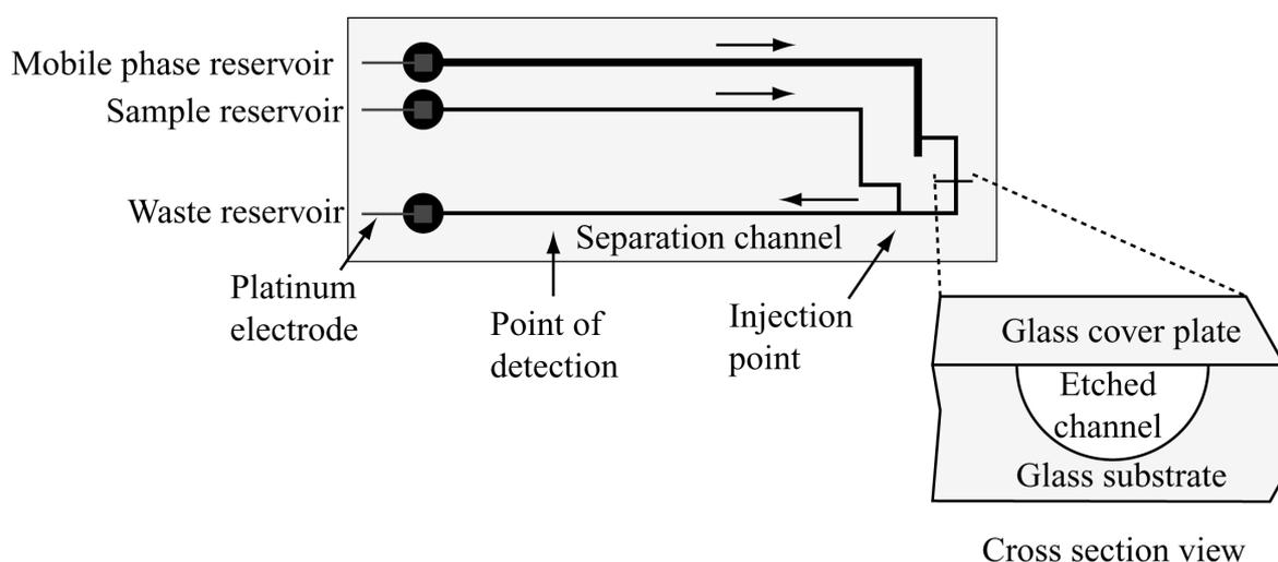
*Figure 5. Example of a CE system etched in a planar glass substrate. The figure shows the construction used in the very first CE on-chip published in 1992 [45]. The substrate was 5 mm thick and the channels were 10  $\mu\text{m}$  deep to which another glass substrate was attached (in a process called bonding). Access holes were drilled in the cover plate and used as buffer reservoirs and insertion of platinum electrodes.*
