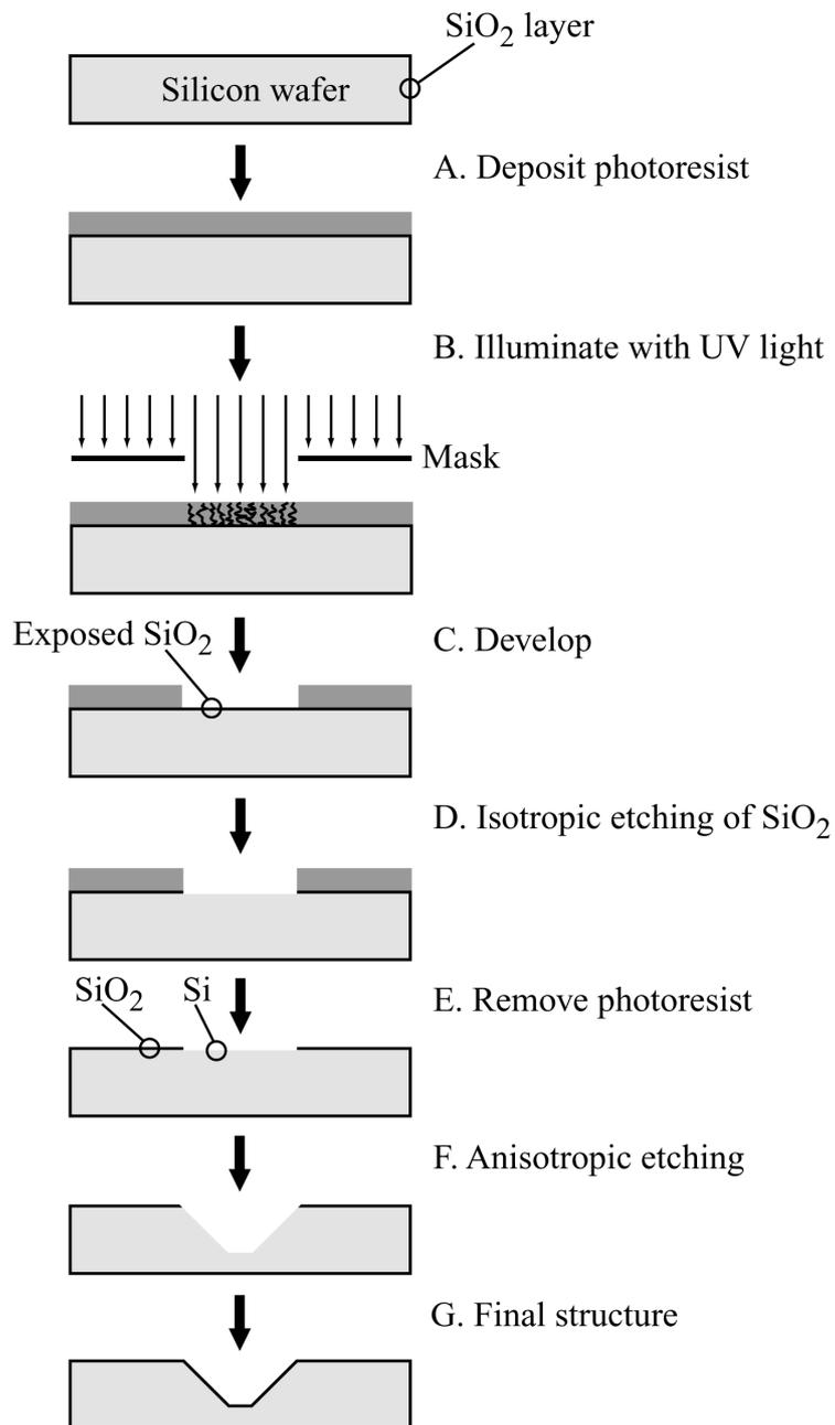
Figure 9. Schematic carton of the machining procedure performed for construction of the silicon microchips used in this thesis. See text for details.
