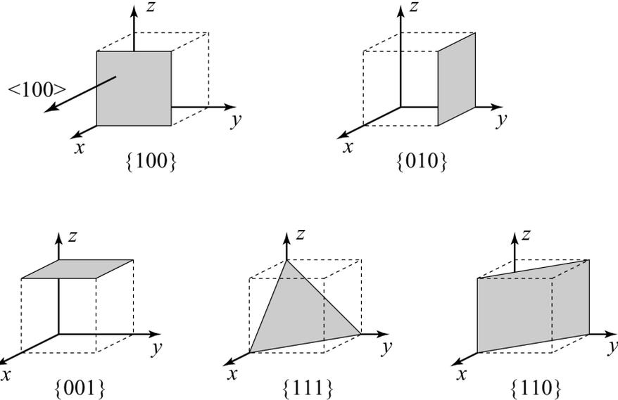
Figure 8b. The different crystal planes, which describes mono-crystalline silicon. For some wet etching solutions the silicon crystal behaves anisotropic, and it has been found that  $\{110\}$  is usually the most rapidly etched plane, while  $\{100\}$  is intermediate and  $\{111\}$  the slowest.
