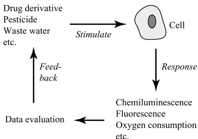
*Figure 4. General principle for a cell-based assays set-up. The analyte can be drug derivative, pesticide or wastewater and depending on the cell type used it will respond by different means. The obtained read-out is then correlated back to the stimulation, and depending on the set-up, information such as toxicity, biological activity or bioavailability can be obtained.*
