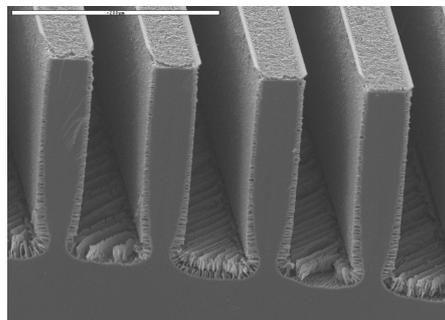
*Figure 11. SEM image of a silicon microchip with porous surface: This microchip structure was used as immobilisation support for antibodies (paper I and II) and enzymes (paper III and IV). The channels were 235  $\mu\text{m}$  deep, 25  $\mu\text{m}$  wide and 10 mm long. Each chip had 42 channels, which in each end fall into inlet and outlet basins, with a total volume of approximately 4.7  $\mu\text{l}$ .*
