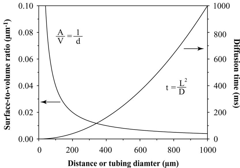
*Figure 7. Plots showing the surface-to-volume ratio (combination of Equation 3 and 4) and diffusion time (Equation 2, for a species having a diffusion coefficient of  $1 \times 10^{-6} \text{ m}^2/\text{s}$ ) as functions of distance. The most common interior channel dimensions in microfluidic systems range approximately from 200 to 10  $\mu\text{m}$ .*
