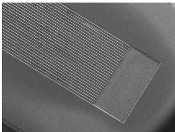
*Figure 15. Microchip construction used as support for immobilising living cells (paper IV and V), consisting of 28 parallel V-grooves, 10 mm long, 100  $\mu\text{m}$  wide at the top and 71  $\mu\text{m}$  deep, with each end falling into inlet and outlet basins. The total volume was approximately 1.9  $\mu\text{l}$ .*
