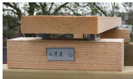
Figure 7. Test set up for reference detail of spruce board (cross section 22x95 mm 2 )
