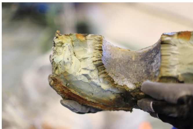
Figure 32. Excavated bentonite sample of Deponit CA-N from the ABM2-experiment. Visually dark corrosion products at the heater interface and white centrosymmetrical precipitates some centimeters away can be observed.
