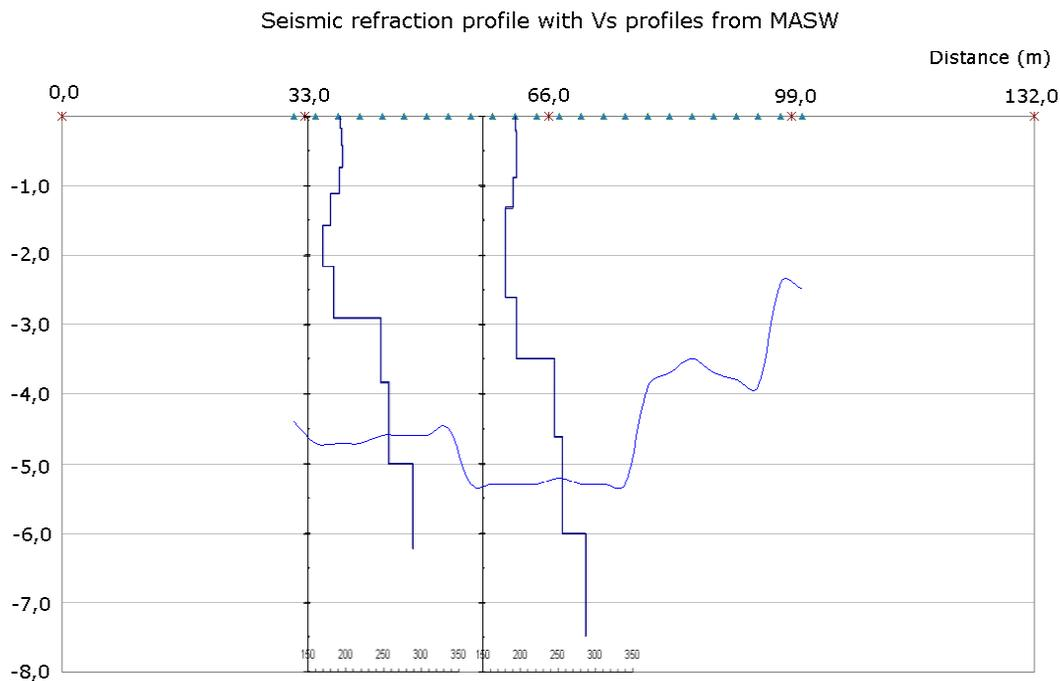
Figure 3. Superposition of Vs soundings to seismic refraction profile (the vertical line indicates the place the Vs model is attributed to).
