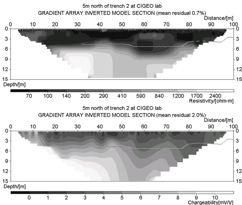
Figure 2. Inverted geoelectrical sections with depth to refractor from seismic survey marked: resistivity (top) and induced polarisation (bottom).
