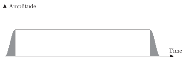
Figure 2.6: Pulse shaping using the raised-cosine function. The gray parts of the signal indicate the extensions.
