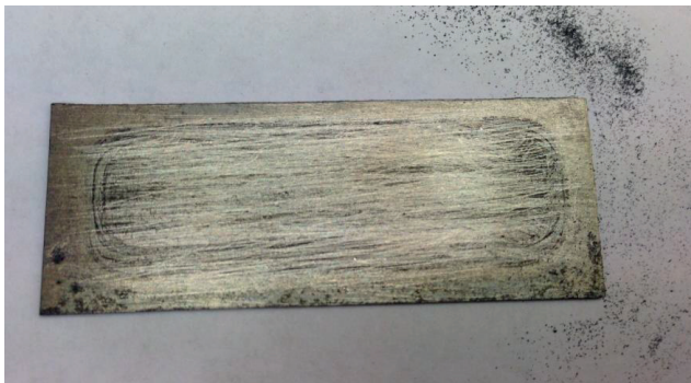
Fig 7.9: This picture shows the appearance of the yttrium foil from fig 7.8 after mechanical removal of green dissolved yttrium material. Less than 1 % mass weight was removed.
