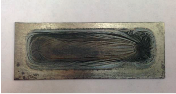
Fig 7.8: A direct water cooled yttrium foil ( 50 \times 20 \times 0.64 \text{ mm}^3 ) irradiated with 45 \mu\text{A} protons for 3 h.
