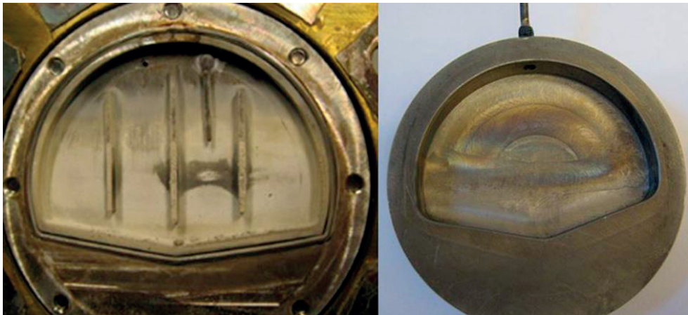
Fig 6.6: The old silver target (left picture) with support bars clearly suffers from silver colloid problems originating from the deterioration of the silver because of the proton beam power. The first Nb-body (right picture) was intact even after 8 months of daily productions
