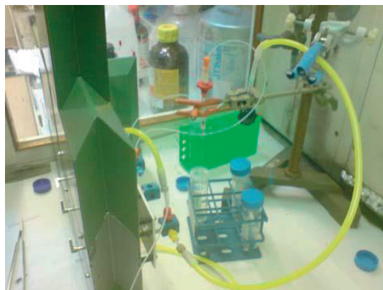
Fig 7.10: Manual separation of ^{89}\text{Zr} from ^{89}\text{Y} foils in Lund.
