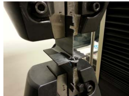
Figure 7. Specimens attached to the tensile machine.
