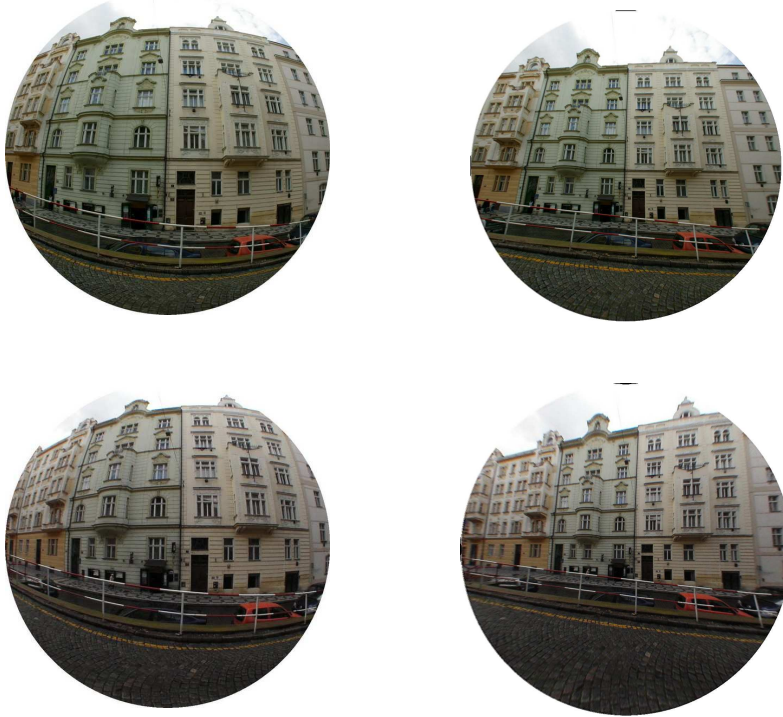
Figure 8.5: Real data, 60% cutouts from omnidirectional images. (Left) Input images with different radial distortions for camera 1 (Top) and camera 2 (Bottom). (Right) Corrected images.
