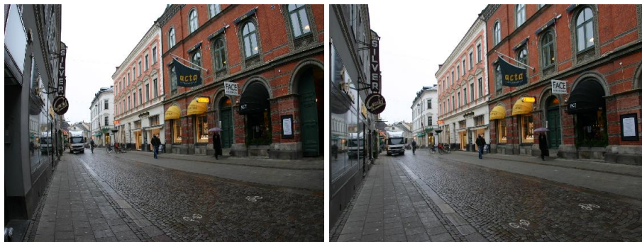
Figure 10.1: Left: An image taken with a fisheye lens. Right: The same image rectified when kernel voting is used to determine the radial distortion
