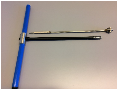
Figure B4. 2. Tree core drill and collected tree drill core.
