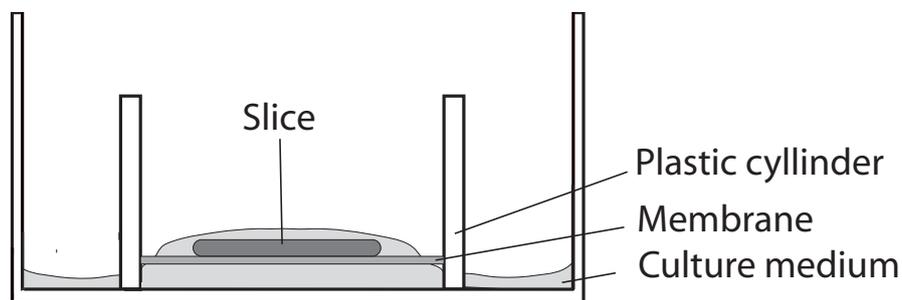
**Figure 4.** The interface method for culture of tissue slices. The slice lies on a porous membrane between the culture medium and air.
