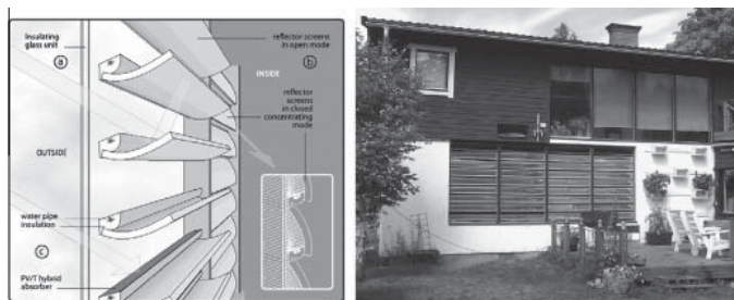
Fig. 1. Left: the solar window with water cooled PV cells, tiltable reflectors and anti-reflection treated glazing. Right: the solar window in Solgården.
