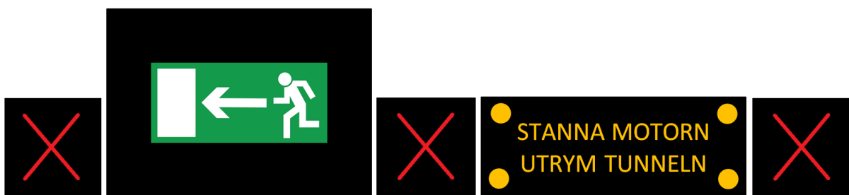
Figure 4. Recommended TIS design.
