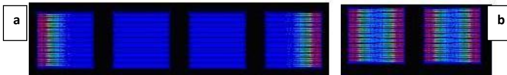
Figure 2: Schematic representation of sample build up for scan length studies, scan length of a) 50mm b) 10mm
