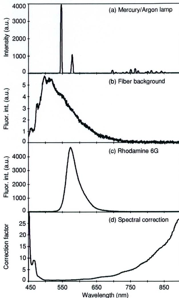
**Figure 2.** (a) Recording of the emission spectrum of a mercury/argon lamp (integration time 10 ms). (b) Laser-induced intrinsic fiber fluorescence level to be subtracted from recorded spectra (intensity scaled for 10 ms integration time). (c) Fluorescence spectrum from a Rhodamine 6G solution (integration time 10 ms). (d) Spectral correction curve.
