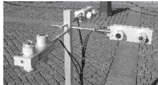
Fig 1. Instrument setup for measuring short- and long wave radiation fluxes from six directions (downward, upward, north, east, south, west) [16]
