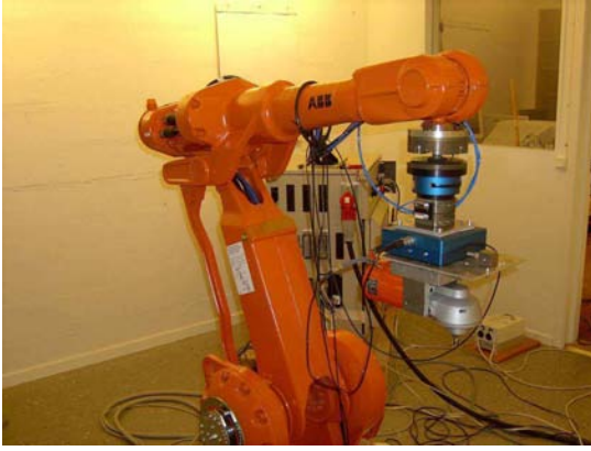
Fig. 2. The experimental setup. An ABB industrial robot IRB 2400 with an open control architecture system is used. The wrist sensor is placed between the robot tip and an compliance tool where the grinding tool is attached. The accelerometer is placed on the tip of the grinding tool.
