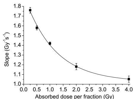
**Figure 4.** The slope of the dose response for the various fractionation schemes versus the dose per fraction for the nMAG dosimeter (2% MAA). The approximately linear regions in the low dose area of R2 versus absorbed dose curves were used when the slopes were estimated. Further, the uncertainty bars correspond to 1 SD of the linear fits from which the slopes were obtained. The exponential curve was included in the figure as a visual aid.
