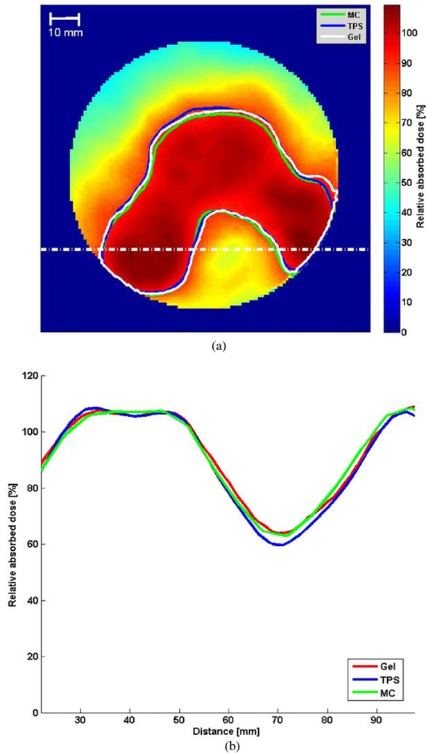
**Figure 2.** (a) Color map of the relative absorbed dose calculated by the TPS. The overlaid 90% isodose lines are extracted from the gel measurement (white line), MC simulations (green line) and TPS calculations (blue line). Profiles extracted across a region with steep dose gradients, along the white dotted line in (a). The profiles correspond to the gel measurement (red line), the MC simulation (green line) and the TPS calculations (blue line).
