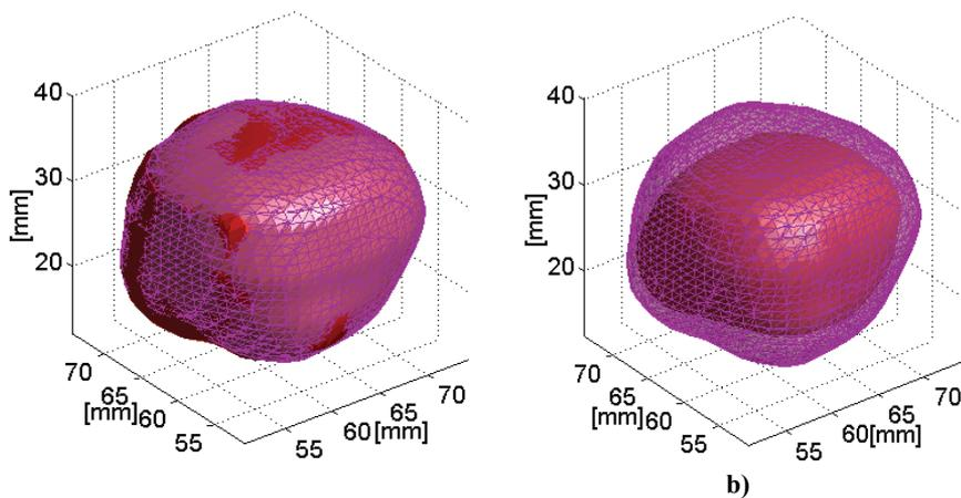
**Figure 22.** The 90% isodose surface overlay of the gel measurements obtained in static mode (wire framed pink volumes) and gel measurements obtained during motion (red volumes). The good agreement between the static and tracked measurements is presented in **a)**. The smaller red non-tracked volume in **b)** visualizes the reduction of the 90% isodose volume due to motion.
