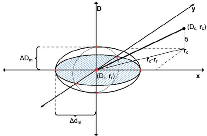
**Figure 12.** An illustration of the  $\gamma$  index concept. The reference dose and position is denoted by  $(D_r, \mathbf{r}_r)$  and the compared dose and position is denoted by  $(D_c, \mathbf{r}_c)$ . The ellipsoid represents the given acceptance criteria. (Drawing by Sacha af Wetterstedt)
