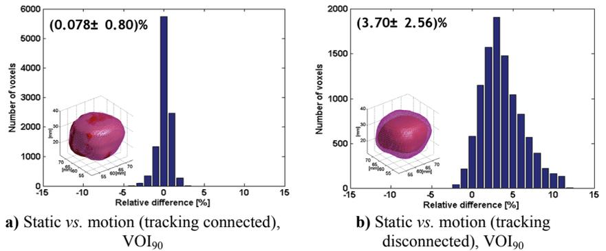
**Figure 23.** The distribution of voxel-by-voxel deviations between the different gel measurement sets within the volumes enclosed by the 90% isodose surface. The number of voxels is plotted against the difference in relative dose between the two analyzed volumes. Note the different scale of the ordinates.
