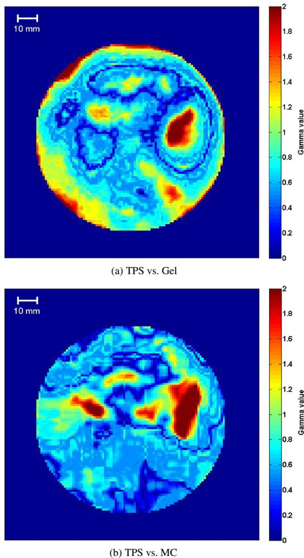
**Figure 5.** 3D-gamma map resulting from the 1%/2 mm evaluation. The cluster of gamma failures was found 15–20 mm from the isocenter within the volume enclosed by the 90% isosurface. In the TPS versus gel evaluation (a), additional gamma failures along the gel container surface are observed. These deviations could probably be attributed to the setting of the gel.
