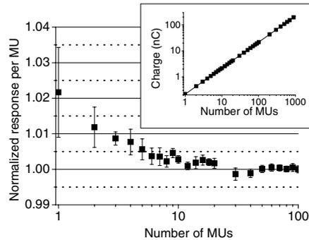
**Figure 1.** The response per monitor unit versus the number of monitor units for the 18 MV beam, Elekta Sli, normalized to the 100 MU measurement. A minimum of 23 MUs, 0.25 Gy, per beam was used. The uncertainty bars represent the spread from repeated measurements (1 SD).
