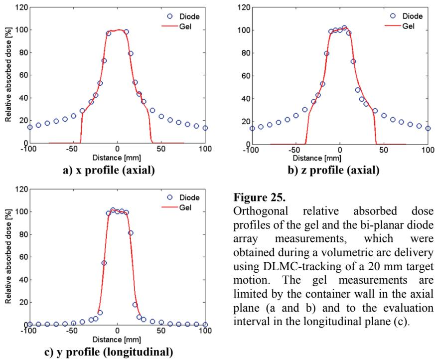
**Figure 25.** Orthogonal relative absorbed dose profiles of the gel and the bi-planar diode array measurements, which were obtained during a volumetric arc delivery using DLMC-tracking of a 20 mm target motion. The gel measurements are limited by the container wall in the axial plane (a and b) and to the evaluation interval in the longitudinal plane (c).
