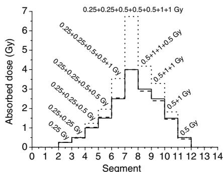
**Figure 6.** A simulated example of absorbed dose profiles for the nMAG system with 2% MAA. The figures in the graph denote the hypothetical fractionation scheme for the segments of the absorbed dose profile. The solid line represents the true absorbed dose. The absorbed dose profile obtained using gel vial calibration (method I, dotted line) was compared with the absorbed dose profile obtained using a relative calibration (method II, dashed line).
