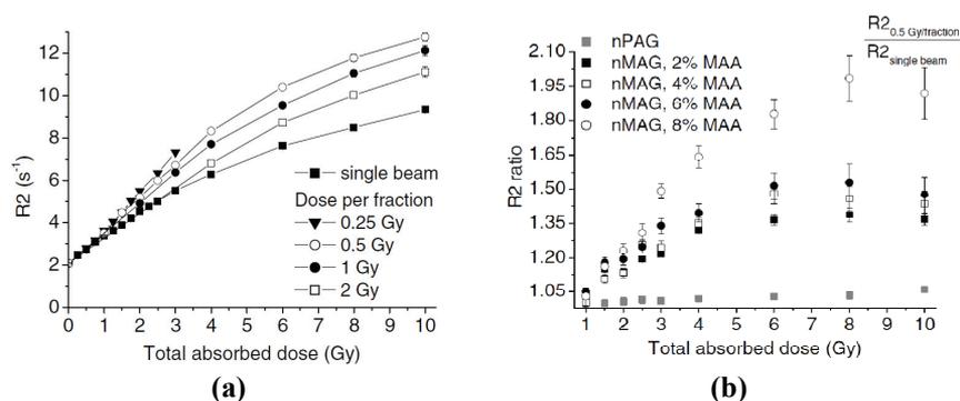
**Figure 13 a)** R2 dose response for nMAG samples (2% MAA) irradiated to absorbed doses of up to 10 Gy. When the total dose was delivered in sequential beams the R2 dose response for the total absorbed dose increased with increased number of beams. **b)** The effect of different amount of MAA, normalised to a single dose irradiation. Corresponding nPAG data is included for comparison.
