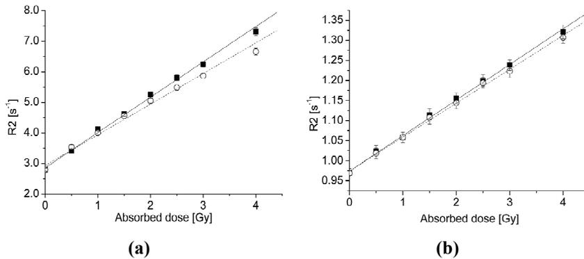
**Figure 14.** R2 dose response for **a)** nMAG and **b)** nPAG vials irradiated to absorbed doses up to 4 Gy. Two sets of samples for each gel were irradiated during a single beam delivery (empty circles) or during gated delivery with 12 MU every 6.5 s (black squares).
