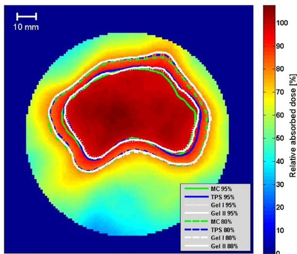
**Figure 1.** Color map of the relative absorbed dose calculated by the TPS in a slice away from the normalization volume. The overlaid 80% and 95% isodose lines are data from the two gel measurements (white lines), MC simulations (green lines) and TPS calculations (blue lines).
