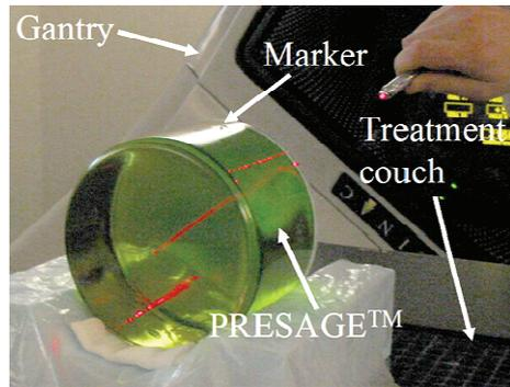
**Figure 8.** The Radiochromic plastic 3D dosimeter. Photo Courtesy of Mark Oldham, Duke University Medical Center.
