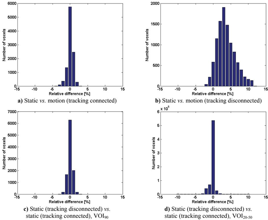
**Figure 3.** The distribution of voxel-by-voxel deviations between the different gel measurement sets within the volumes enclosed by the 90% isodose surface, a) - c), and the volumes enclosed by the isodose surface interval 20-50%, d). The number of voxels is plotted against the difference in relative dose between the two analyzed volumes. Note the different scale of the ordinates.
