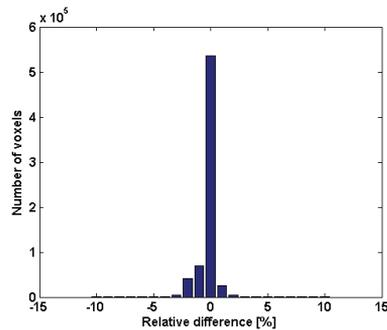
**Figure 24.** Static (tracking disconnected) vs. static (tracking connected), VOI<sub>20-50</sub>. The distribution of voxel-by-voxel deviations between the different gel measurements within the volume enclosed between the 20% and 50% isodose surfaces. The number of voxels is plotted against the difference in relative dose between the two analyzed volumes.
