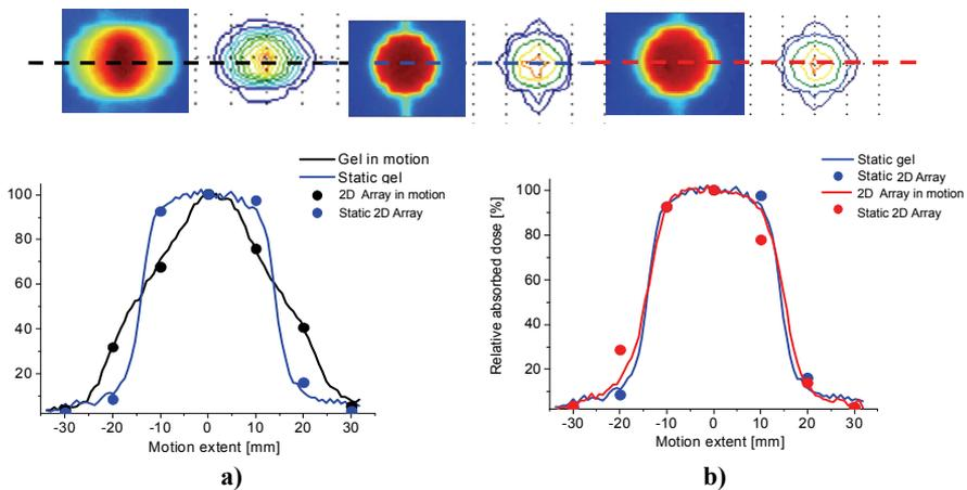
**Figure 17.** Relative absorbed dose profiles extracted from nPAG (lines) and 2D ion chamber array (dots) measurement data, performed with the detectors in motion or in a static position a) Tracking system disconnected. Detector moving (black) and in a static position (blue). b) Tracking system connected. Detector moving (red) and in a static position (blue).
