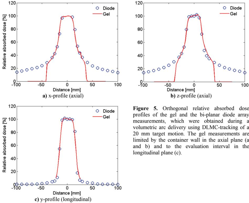
**Figure 5.** Orthogonal relative absorbed dose profiles of the gel and the bi-planar diode array measurements, which were obtained during a volumetric arc delivery using DLMLC-tracking of a 20 mm target motion. The gel measurements are limited by the container wall in the axial plane (a and b) and to the evaluation interval in the longitudinal plane (c).
