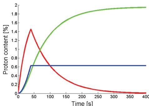
**Figure 10.** An illustration of how the proton content in each compartment varies during time. When irradiation starts the protons in P1 are transferred to P2 (red curve) and further to P3 (green curve). During irradiation protons are also transferred from P2 to P4 (blue curve).
