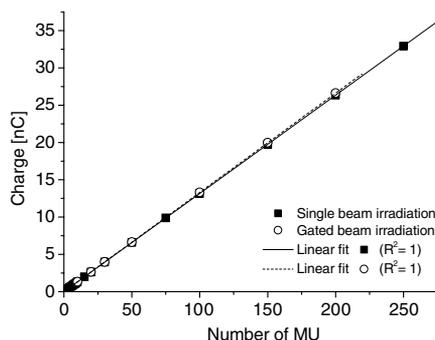
**Figure 2.** The accumulated charge in the gating mode compared to the charge collected from single beam irradiation. The gated irradiation was delivered in fractions of 10 MU/beam-on in the gating mode. Uncertainty bars represent the spread from repeated measurements (1 SD) and are smaller than the symbols and therefore not visible.
