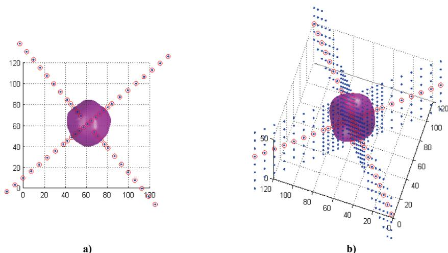
**Figure 1.** The purple volume corresponds to the gel measurement ( $VOI_{50}$ ) and the blue dots denotes the location of the diodes within the Delta<sup>4®</sup>. The red circles point out the diodes whose measurements are compared with the gel measurement. In the view a) are the diode boards within the Delta<sup>4®</sup> easy to recognise. In b) a tilt of the a) is presented. The gel measurement cover the part of Delta4<sup>®</sup> with the highest resolution (5 mm)
