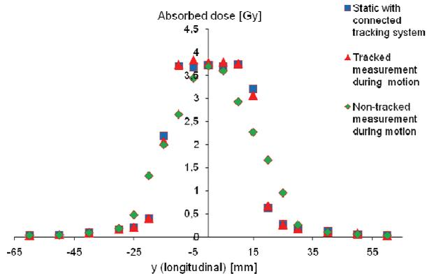
**Figure 4.** Absorbed dose profiles through the isocenter of the Delta<sup>4®</sup> detector. Data from three measurements are presented: non-tracked delivery during motion (green dots), tracked delivery during motion (red dots) and static delivery with the tracking system connected (blue dots).
