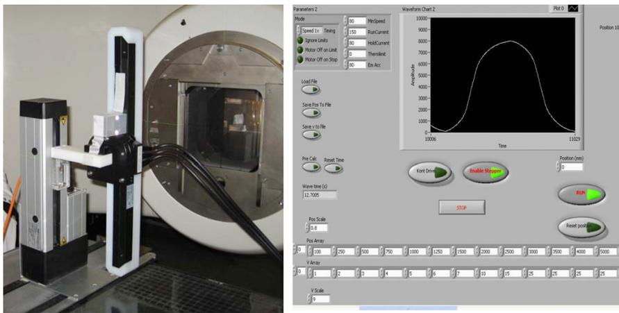
**Figure 1.** The robot simulated the respiration motion, here shown with the LDA detector attached to the moving platform (left). The RPM system (Varian) was used to monitor the position of the platform. The motion was generated using a step motor, controlled by an in-house-developed software (right) in which the motion parameters such as amplitude, frequency and curve pattern were defined.
