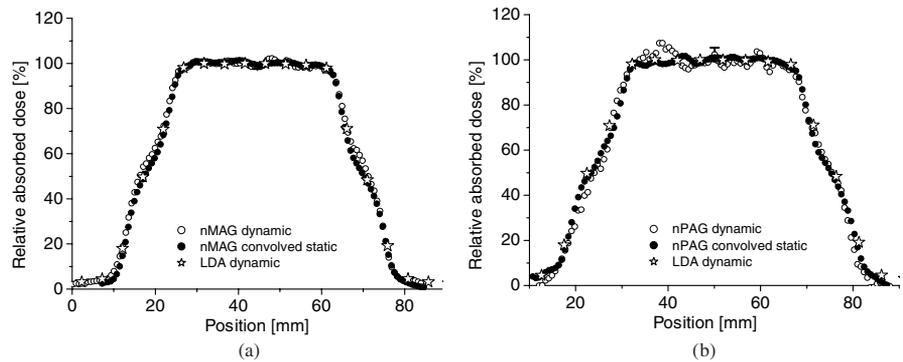
**Figure 3.** Relative absorbed dose profiles from the (a) nMAG and (b) nPAG during respiratory-like motion in and out of the beam. The uncertainty bar in the dynamic gel data corresponds to 1 SD of the relative absorbed dose in the flattened area. In the nMAG case, the uncertainty bar is of the same magnitude as the symbols and therefore not visible.
