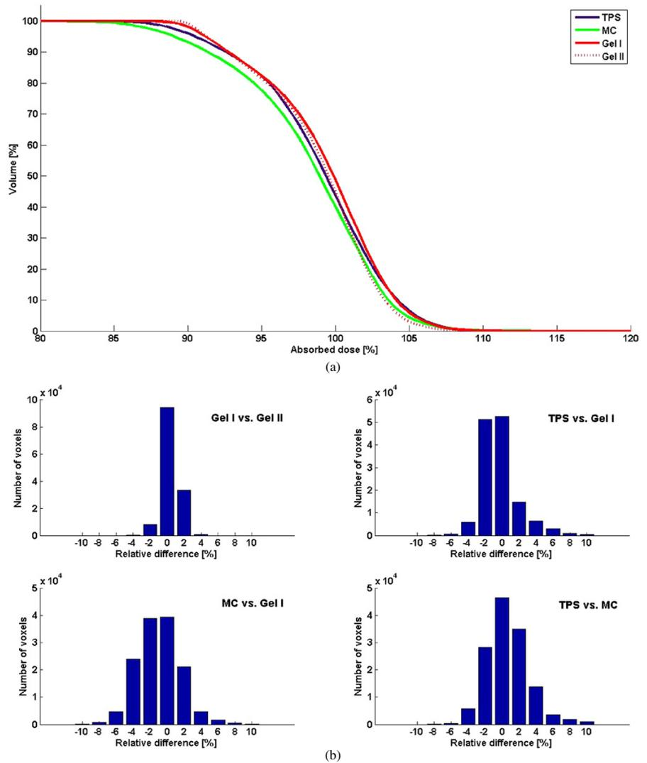
**Figure 4.** (a) RapidArc™ TPS plan MC-calculated and gel-measured cumulative dose volume histogram (DVH) for the 90% isodose volume. (b) The distribution of voxel-by-voxel deviations between the different datasets within the volumes enclosed by the 90% isodose surface. The number of voxels is plotted against the difference in relative dose between the two analyzed volumes. Note the different scale of the ordinates.
