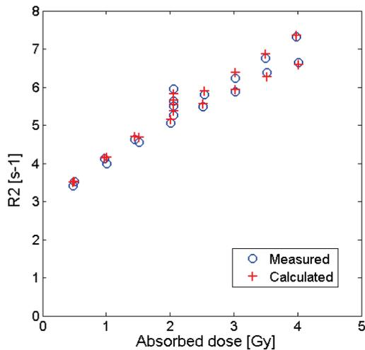
**Figure 18.** The difference between calculated R2 values (red crosses) and measured R2 values (blue circles) was on average  $1.1 \pm 1.6\%$  (1SD) for the experiments with nMAG gels irradiated with different fractionation patterns.
