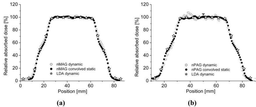
**Figure 15.** Relative absorbed dose profiles from the (a) nMAG and (b) nPAG during respiratory-like motion in and out of the beam (empty circles). Also included is corresponding LDA data (stars) and convolved data (black circles).
