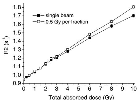
**Figure 3.** R2 versus the total absorbed dose for the nPAG (3%AA/3%BIS). The lines were included as a visual aid. The uncertainty bars correspond to 1 SD in the R2 map. In most cases the uncertainty bars were smaller than the symbols and therefore not visible.
