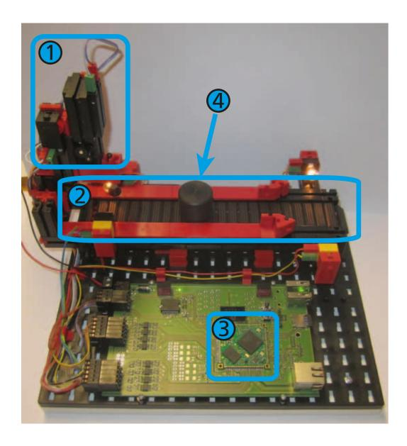
The OPC UA support was tried out on a physical device in an Industry 4.0 setting. The device consists of a punching machine (1) and a conveyor belt (2). A microcontroller (3) was used to expose the device as variables in an OPC UA server.
