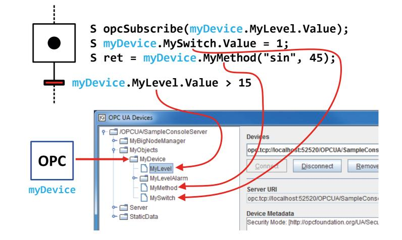
An OPC UA Object is bound to a node in an OPC UA server. The OPC UA variables and methods are then used like native variables and methods.
