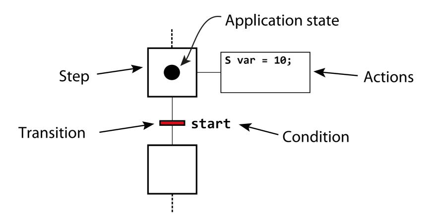
Grafchart is a graphical programming language based on the PLC standard language SFC. The basic building blocks are steps (application states) with actions (what to do when) and transitions (how and when to change application state).
