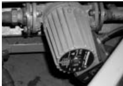
Figure 73: The Water pump used in the fuel cell bus.
