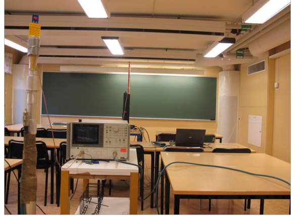
Fig. 1. Overview of the measured scenario. Tx antenna in front and Rx antenna in the back.
