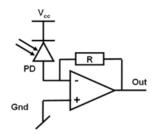
Fig. 3.2.1. Simplified configuration for high speed photo diode configuration. Impinging light displaces the IU curve towards negative currents (See Fig. 3.1.7).
