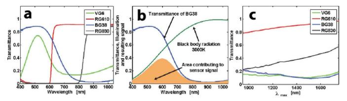
Fig. 4. (a) Transmission spectra of four commercial Schott colored glass filters expressed in wavelengths. (b) Illustration of transmitted light from a blue glass filter when illuminated by a 3000 K black-body; the shaded area represents the resulting signal received by the camera according to Eq. (1). (c) Transmitted light versus black-body peak radiation (inversely proportional to temperature), with each spectral value arising from a different temperature.
