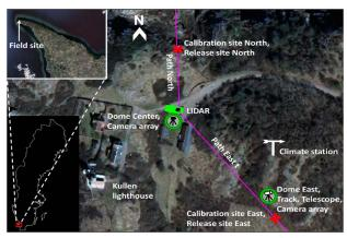
Fig. 1. (Color online) Photographic setup overview of the field site at Kullaberg and its location in Sweden. The site has the coordinates N 56° 18′, E 12° 26′. Shown are the locations of the lidar equipment, the center dome in which the IR cameras were installed, the east dome with the passive telescope, and a weather station. Also shown are two directions in which different lidar measurements were performed.
