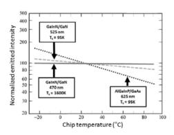
Fig. 3.1.4. Thermal dependence of the emissive yield of LEDs. Red LEDs are more susceptible to temperature changes than blue LEDs. This is an important detail in analytical applications. Data from Toyoda Gosei Corp. 2004
