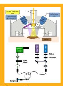
Schematic diagrams of the two spectrometers showing the steady state spectrometer measurement head (top) and the optical layout of the time-resolved system (bottom).
