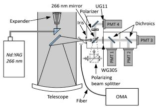
Fig. 2. (Color online) Schematic overview of the fluorescence and polarizing lidar system. The light from the laser is expanded and variably diverged before it is sent out vertically or in other inclinations. The returning light is focused onto the detector system with a 40 cm diameter telescope. Here it is separated into different spectral bands or two polarization directions, or it is sent through a fiber to an OMA.
