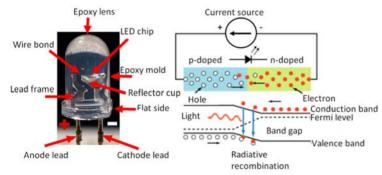
Fig. 3.1.1. Left: common epoxy casing of LEDs. The expoxy serves both for stabilizing the parts, focusing and index matching. The chip is placed in a reflecting cup, which is also the cathode lead. Right: Common diagram in solid state physics showing a representation of the potential energy drop in a LED bandgap. Public domain images adapted from Wikipedia.org.
