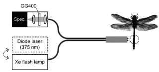
Fig. 5. Setup for fiber point measurements. Either a UV laser line or white light is passed into the bifurcated probe. The sample geometry is maintained constant between the measurements. A longpass GG400 filter prevents blooming in the spectrometer (Spec.).
