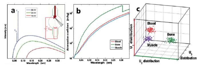
Fig. 1. (a) X-ray tube and three bremsstrahlung spectra generated by different tube voltages (adapted from Ref. 2). (b) X-ray attenuation spectra for different substances (data from Ref. 3). (c) Location of data points from several objects in an x-ray color space expanded by several tube voltages.
