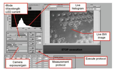
FIG. 5. (Color online) Graphical user interface (GUI) for controlling the LabView software. The GUI includes a live monochrome preview, live histogram, and settings can be made for the LEDs and camera. The settings can be added to a measurement protocol, which can then be executed automatically.
