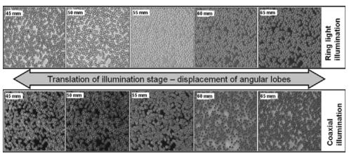
Fig. 4.4.4 The concept of numerical aperture becomes slightly more complicated when using reflecting microscope objectives. Similar discussion arises in relation to form factors of reflective telescopes. Above the effect of translating the illumination stage, and thus the impinging angles, in P3 is apparent, bright field becomes dark field and visa versa. The pictures depict a thin blood smear and are all acquired at the yellow wavelength 590 nm.
