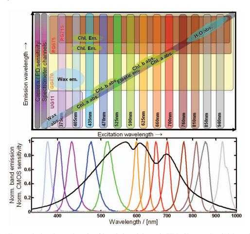
FIG. 2. (Color online) Upper panel: schematic spectral overview of the excitation emission matrix (EEM) with common botanical chromophores. Lower panel: Wavelength of LED emissions and the CMOS camera sensitivity (black curve).
