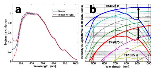
Fig. 3. (a) The absolute filament temperature is determined by minimizing the variance among the system transmission spectra, which are know to be the same. (b) Computed and actual filament emissions spectra on a log scale. (Equidistance at different temperatures is indicated by the arrows at a particular wavelength, showing that the system transmission measured for the two temperatures is the same—it is a system invariant.)
