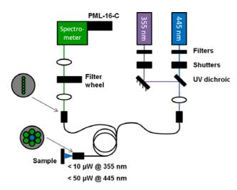
**Figure 2** (online color at: www.biophotonics-journal.org) Experimental layout of the fluorescence lifetime fibre probe spectrofluorometer (instrument B).
