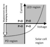
Fig. 3.1.7. LEDs can in general operate in different regimes: As LEDs, as Photodiodes, or as Photovoltaics. The regime is determined by the quadrant in the UI characteristics where the operation point is. P denotes the power consumed by the device.
