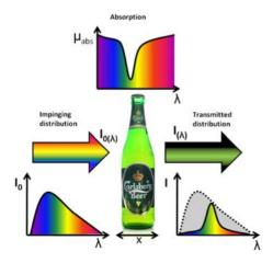
Fig. 2.5.2. The Beer Lambert law describes the exponential decay of intensity for light propagating in an absorptive medium. The decay arises due to the constant survival chance per unit length.
