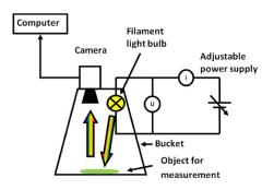
Fig. 2. Setup for Wien shift imaging. A bucket provides optical isolation for the experiment. Simultaneous recording of current and voltage provides an estimation of absolute temperatures.
