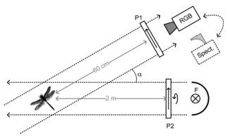
Fig. 2. Setup for color imaging and whole-body polarized reflectance studies. Samples are observed either with a color camera (RGB) or a spectrometer (Spect.) at low angle ( $\alpha=15^{\circ}$ ) through a linear polarizer (P1). Collimated white illumination is provided by a tungsten filament lamp (F) which can be polarized in parallel or perpendicularly to P1 using P2.
