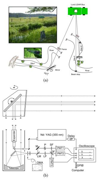
Fig. 1. (Color online) (a) Geographic diagram of the measurement locations. The inserted scenery picture is taken from the indicated position and direction; also shown is a male *C. splendens* damselfly. (b) Key equipment/components of the fluorescence lidar (PMT-1 is for detection of elastic scattering, while PMT-2 and PMT-3 are for yellow and blue bands of fluorescence, respectively).
