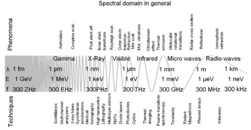
Fig. 4.2.1. Spectral overview showing important terms and technologies in respect to the wavelength of light.
