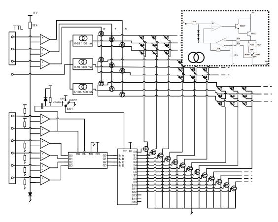
FIG. 4. Electronic schematic used for the multiplexing of sources. Inset: electronic scheme for the adjustable constant-current driver. UV and blue LEDs are driven with currents up to 25 mA, whereas the NIR LEDs can be driven with up to 100 mA.
