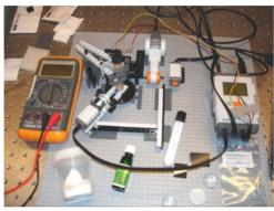
Fig. 4.4.5. Automated polarimetric goniometer made from inexpensive LEDs, film polarizers, LEGO and controlled by a LabView compatible Mindstorm microprocessor. The setup was assembled during an exercise on scattering from powdered milk during a workshop in Lima, Peru<sup>346</sup>.
