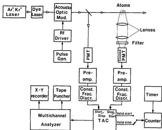
FIG. 3. Experimental arrangement used in the measurements.
