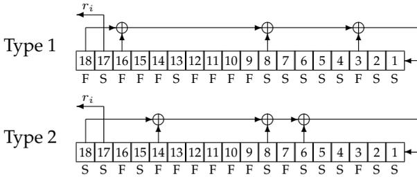
**Figure 6.6:** The jump registers used in Pomaranch Version 3.
