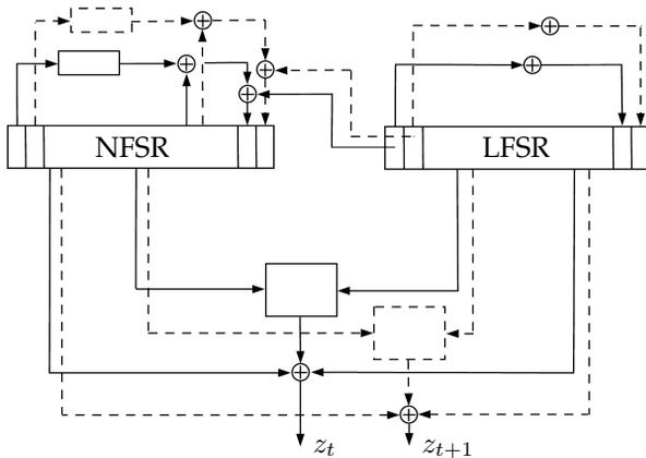
Figure 8.3: Implementation of Grain which outputs 2 bits/clock.
