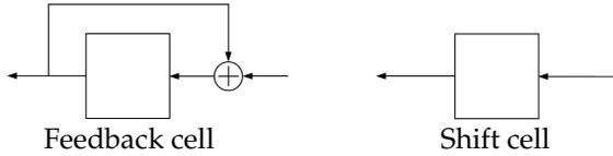
**Figure 6.1:** F-cell and S-cell used in jump registers.
