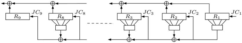
Figure 6.2: Overview of the Pomaranch design principle.
