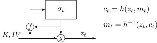
**Figure 2.1:** A model of a synchronous stream cipher.
