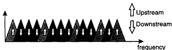
Fig. 1. The Zipper principle of capacity division.
