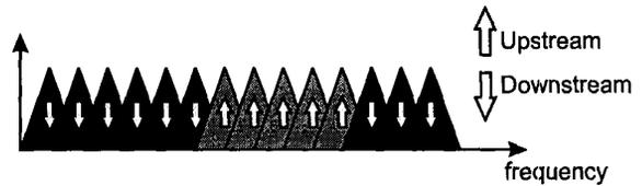
Fig. 3. Sample subcarrier assignment for asynchronous Zipper.
