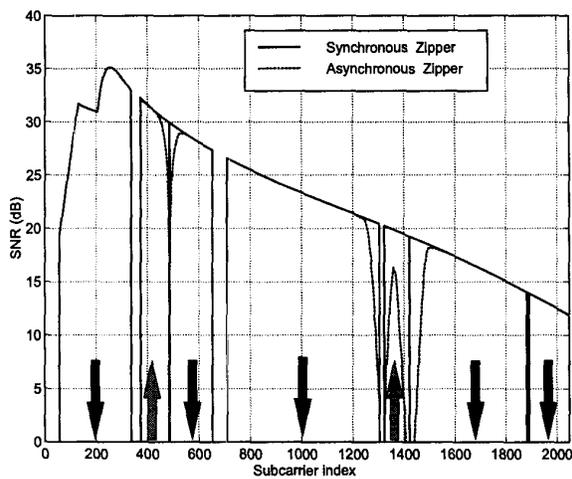
Fig. 8. SNR for asynchronous Zipper compared to synchronized Zipper for an (8:1) asymmetrical case. The arrows indicate the transmission direction.
