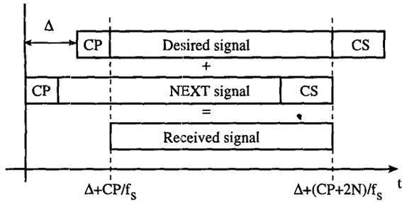
Fig. 2. Timing diagram showing the NEXT symbol frame, the desired symbol frame, and the portion of data extracted from the received frame.
