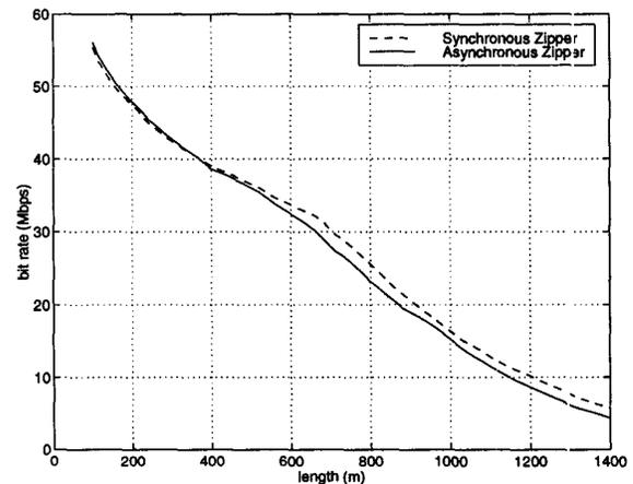
Fig. 10. Downstream bitrate for synchronized and asynchronous Zipper, asymmetrical down/up (8:1) rate.
