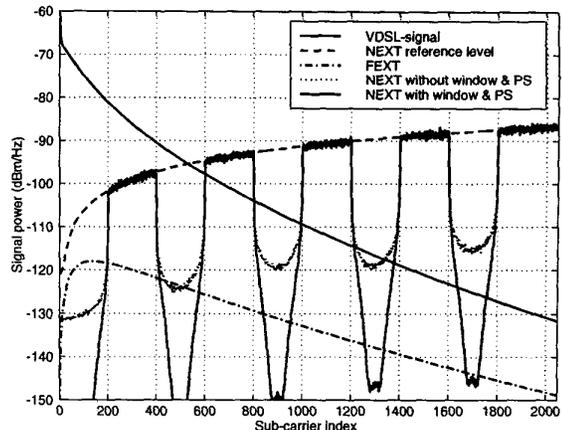
Fig. 7. Suppression of NEXT with and without pulse-shaping and windowing. Every other 200 subcarriers are used upstream.
