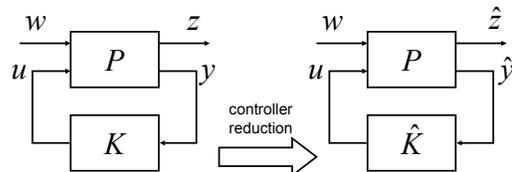
Fig. 1. The block diagram in the left is the feedback interconnection of a plant  $P$  and a controller  $K$ . The problem of controller reduction is to find a lower order controller  $\hat{K}$  to replace  $K$ , so that the performances of the reduced closed loop system (in the right) do not degrade too much.
