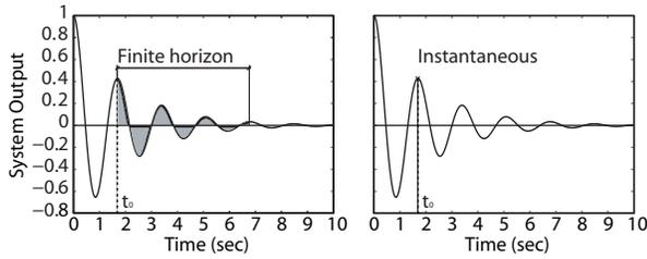
**Figure 2. Finite-horizon (left) vs instantaneous (right) cost measurements**
