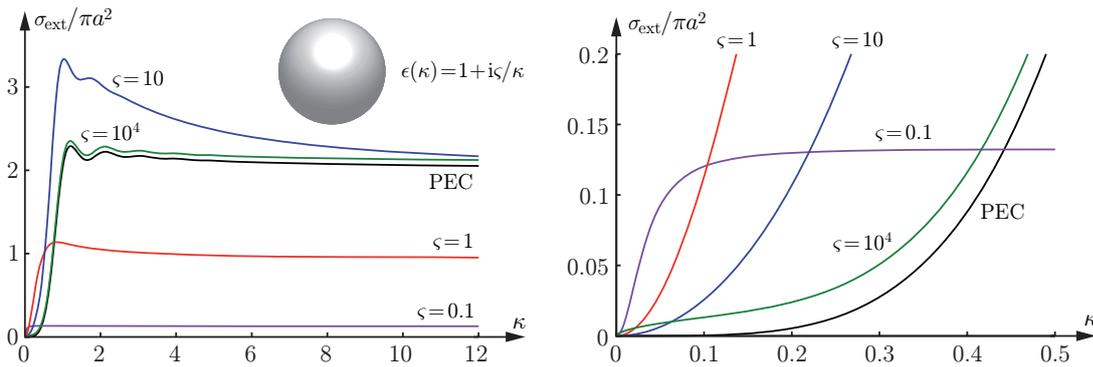
**Figure 1:** The extinction cross section in units of  $\pi a^2$  for a homogeneous and isotropic sphere with  $\epsilon' = 1$ . The right figure is a close-up of the left figure for low frequencies, and as a consequence of (2.4), all curves (except for the one labeled PEC) have the same value of the integral when weighted with  $1/\kappa^2$ .
