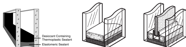
Figure 3.13 Alternative spacer products or “warm-edge” technologies.
