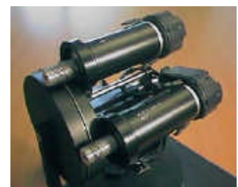
Fig.2. The PHANToM and a close-up of two motors
