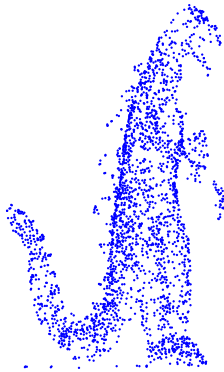
Figure 3: The Oxford dinosaur reconstructed from 2683 point triplets using the method described in this paper. The reconstruction was completed in approximately 2.5 minutes.
