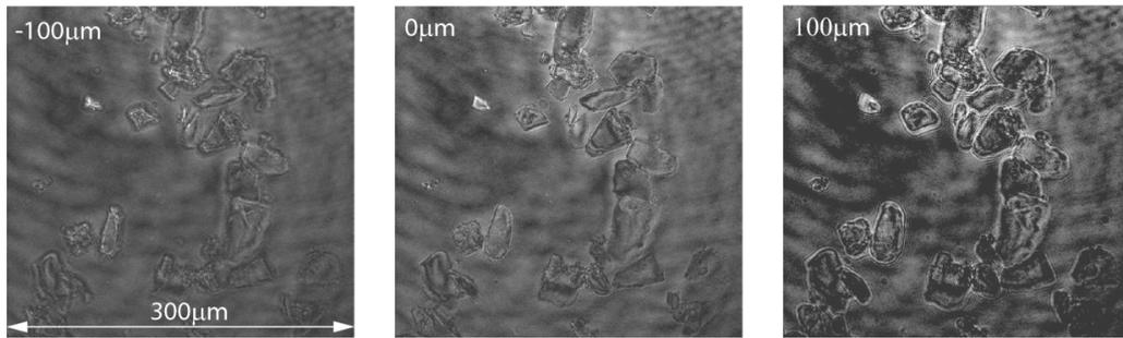
**Figure 3:** Amplitude images of lactose crystals mounted in a liquid with  $n_m = 1.570$ . The Becke lines move out from the crystals into the liquid as the image plane is shifted in the direction of the illuminated wave, *i.e.*, towards the sensor from  $-100 \mu\text{m}$  to  $100 \mu\text{m}$ .
