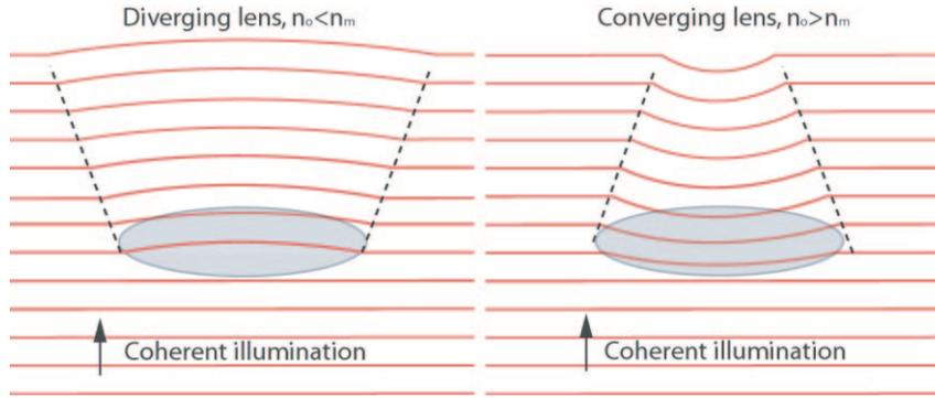
**Figure 1:** Illustrations of the lens effect when a wave impinges on objects with lower and higher index of refraction than the mounting medium. The horizontal lines show the lines of constant phase for the wave field. The phase of an object with low (high) reflective index is advanced (retarded) and if the object is convex it also acts as an divergent (convergent) lens as depicted to the left (right).
