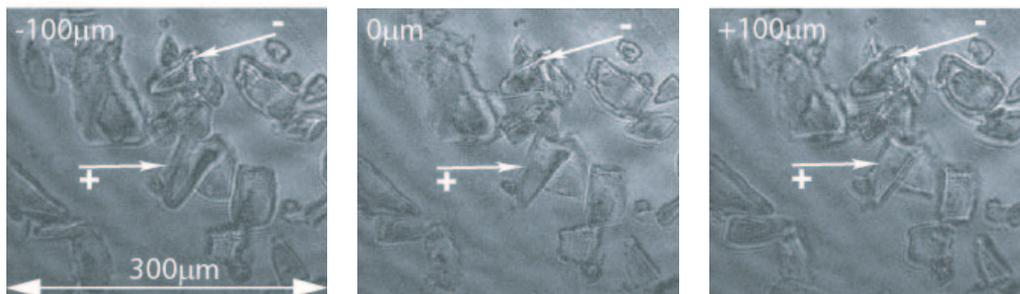
**Figure 5:** Amplitude images of lactose crystals mounted in a liquid with  $n_m = 1.542$ . The Becke lines move into the regions with higher refractive index as the image plane is shifted in the direction of the illuminated wave, *i.e.*, towards the sensor from  $-100 \mu\text{m}$  to  $100 \mu\text{m}$ .
