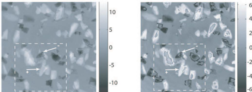
**Figure 6:** Phase images of lactose crystals mounted in a liquid with  $n_m = 1.542$ . The phase increases (decreases) when going from an object with higher (lower) refractive index to an object with lower (higher) refractive index. a) the unwrapped phase image. b) the re-wrapped phase image.
