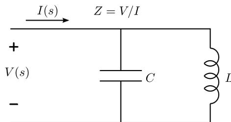
**Figure 1:** The lossless resonance circuit of Example 5.2.
