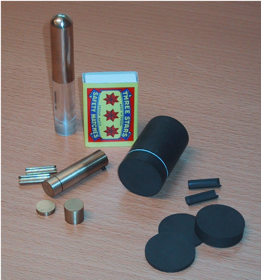
Figure 7. Build-up cap and coaxial phantom used for the measurement of output factors in air. Back left, brass build up cap for BF chambers. Middle front: mini phantom equivalent to the graphite mini-phantom on the right, including bits to surround the stem. Also shown are the disks used to vary the thickness in the beam direction.
