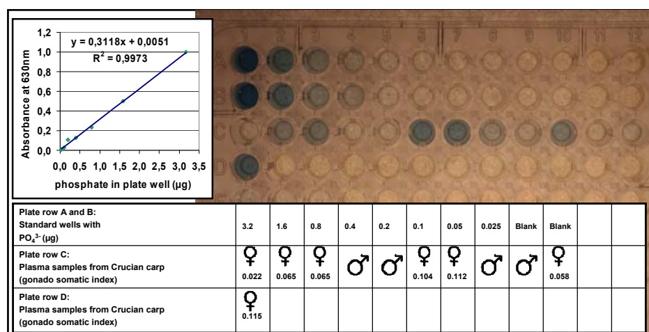
Figure 7. Indirect measurement of vitellogenin by alkali-labile phosphate in plasma samples from Crucian carp. Sample preparation according to Figure 3 and spectrophotometric quantification of phosphate with molybdate and ascorbic acid.
