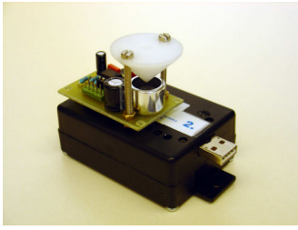
Fig. 1. Stationary sensor network nodes with ultrasound receiver circuit. The nodes are packaged in a plastic box to reduce wear.
