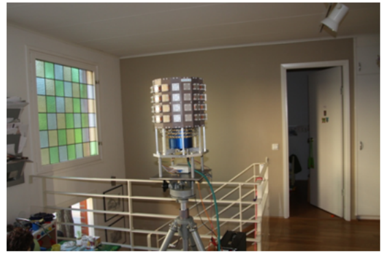
Fig. 3. 128-port receive antenna in the upstairs position.
